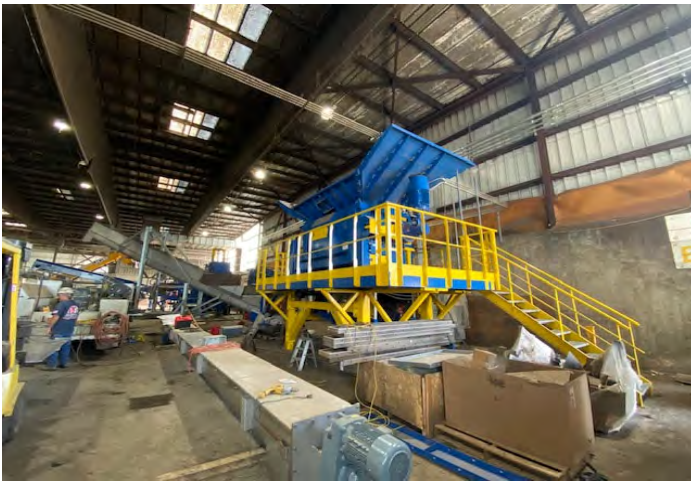
System in-feed / shredder and conveyors
